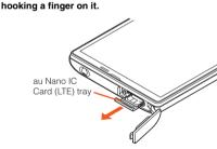
Remove the au Nano IC Card (LTE) from the au Nano IC Card (LTE) tray.
